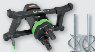
EZR 23 R R/L Set 1.800 W; 200-530 min -1 ; Ø 230 mm; Rührgutmenge 80 kg
