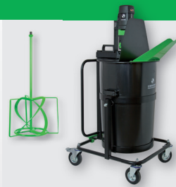
FloorMix 2300 2.300 W; 70/130/160/280 min -1 ; 110 l; Rührgutmenge 150 kg
