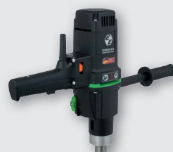
EHB 32/2.2 R R/L 1.800 W; 60-140/200-470 min -1 ; Ø 32 mm in Stahl
